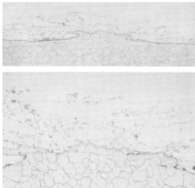
Fig. 13 Transverse section through extruded Tube 10C at site of shrinkage pore in the ID surface of as-cast SS310. Pore was filled in by the molten T-11 and flattened into a low mound during extrusion. Cluster of oxide particles originated in microshrinkage pores surrounding the main pore. Nital etch, 50× (upper), 150× (lower)
